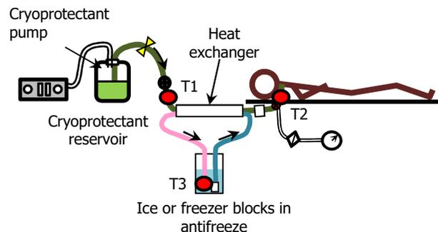
**Figure 2** Old procedure: schematic
