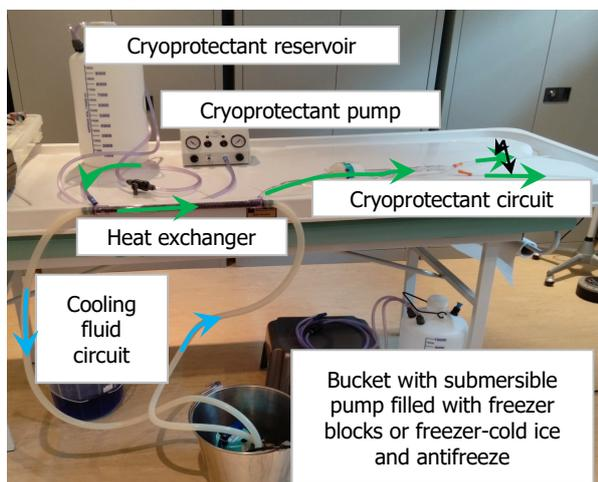
**Figure 1** Old procedure: equipment
