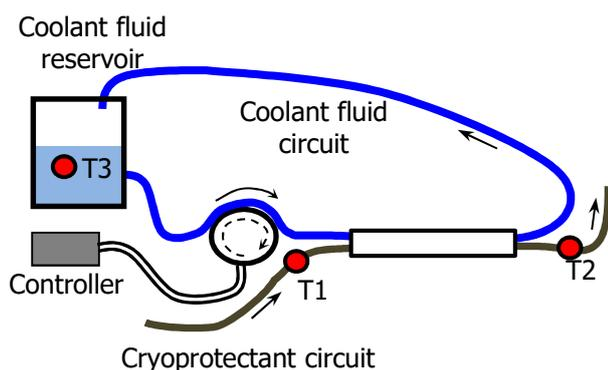
**Figure 3** *New pump circuit*
